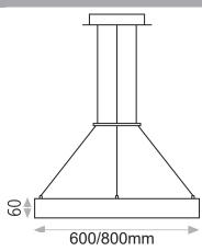
Code LM-3742XXB-8X0 Finishes\*\* Wattage \*\* 55w/75w Lumens 4600lm/5800lm Diam. CCT 3000K Height CRI 80 Width
